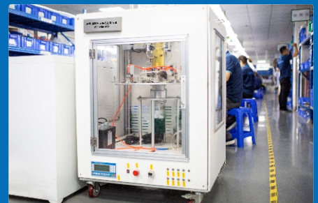
Vacuum test platform
