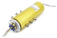
MAPH600S is 6 passages Pneumatic /Hydraulic + 2~96rings Electrical Slip Ring. Connection size including: M5,G1/8", G1/4", G3/8",G1/2" and bigger on request. Electrical rings including power wire, signal wire,Ethernet, USB, Industrial BUS, control Net, and all kinds of sensitive signal, etc. Normally use flange for installation, hollow shaft intallation on request.
