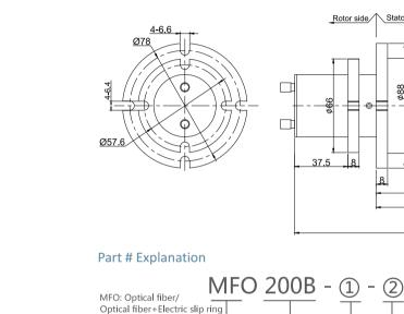
200: 2 channels optical fiber, B type shape
