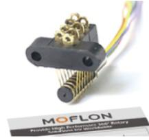
MSP110AC separated slip ring is a type of minitype slip rings. It adopts a separated rotor and contact brushes combination, supporting 10 wires for signal or 1A. The exiting wires in stator and rotor correspondingly 10 colored wires, it can simplify the electrical connection. The 90-degree angle V-groove design has the characteristics of smooth rotation, low torque and low electrical noise, which can exceed ordinary slip ring products.
